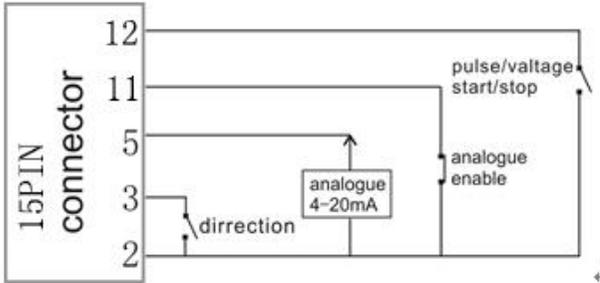
**Note:** Connect Pins 2 and 11 first, speed can be controlled by analogue, direction and S/S are controlled by external signals.
