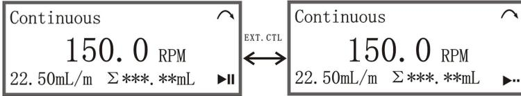
(2) There are 2 ways for external signal to control pump direction and S/S, analog signal controls speed. Connect PIN2 and PIN11 according to “Wiring 3”.
