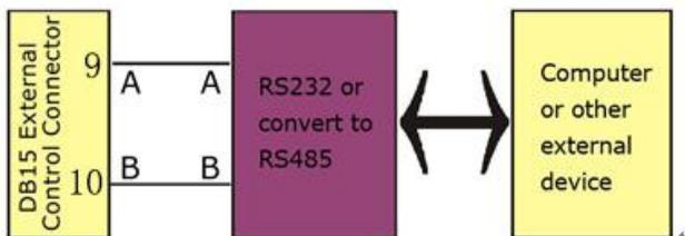
Remote communication control of multiple peristaltic pumps is needed in some applications. The 6/9 pins (A) and 7/10 pins (B) of the external control interface can be connected out according to Wiring 4 above to form the control system as shown in the figure below
