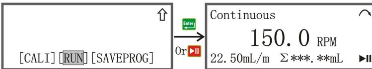
**150.RPM:** The speed at which the pump needs to run, or the speed at which it is set, is generated based on the set flow rate and the number of hoses and hose channels.
