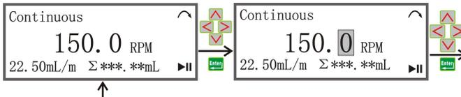
**Note:** ① Invalid adjustment exists due to the flow rate range limited by selected tube size and pump head. ② Flow rate and RPM can be adjusted no
