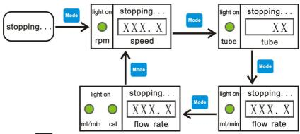
➤ Pressing key can switch between four displays and working modes
