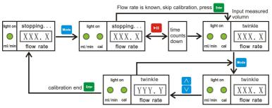
> Flow rate calibration can be repeated. After calibration is
