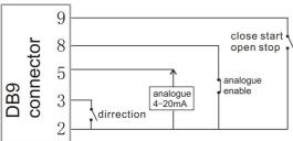
When pins 2 and 8 are connected, running speed is controlled by analogue signals. At this point, apply to pin 5  $\,$  (relative to pin2) a current signal(4 $\sim$
