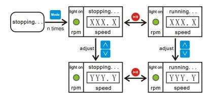
Press the key on the keypad to start the pump, press again to stop.
