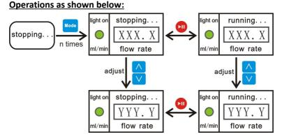
Press the key on the keypad to start the pump, press again to stop.
