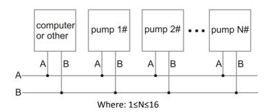
**Note 1:** When there are multiple units, please set up the address number for each unit. It can be controlled through control panel.
